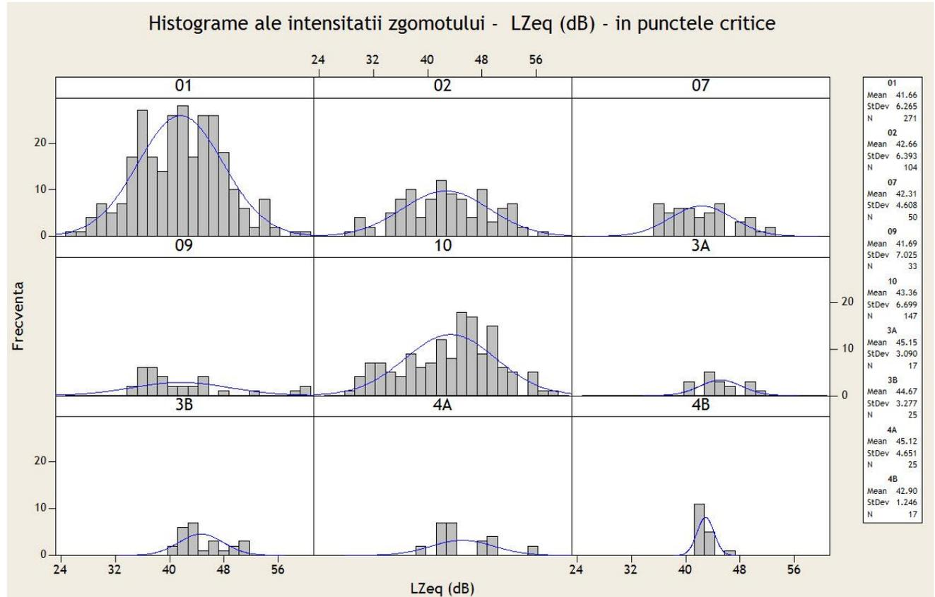
Figure 3.1.B.2 -  $L_{zeq}$  (dB) noise intensity histograms
