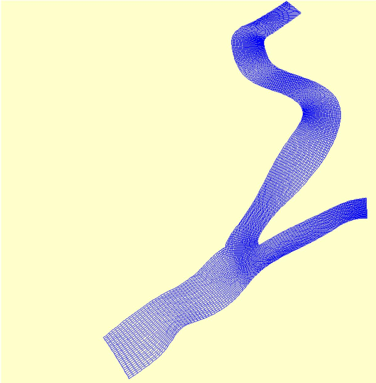
*Figure 3.1.J.4 - Computing network on Bala area*
