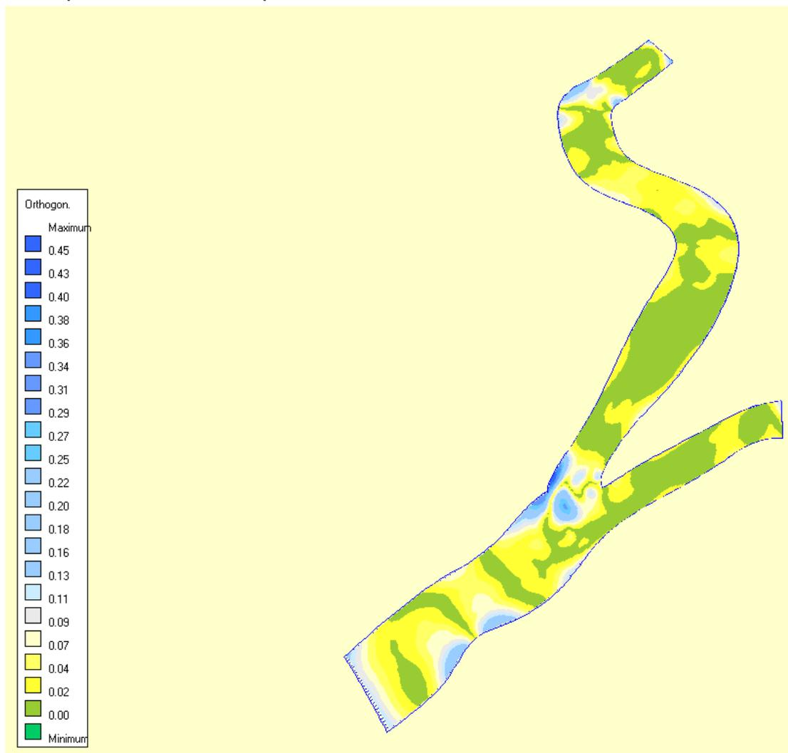
**Figure 3.1.J.6 - Orthogonality analysis for computing network on Bala area**
