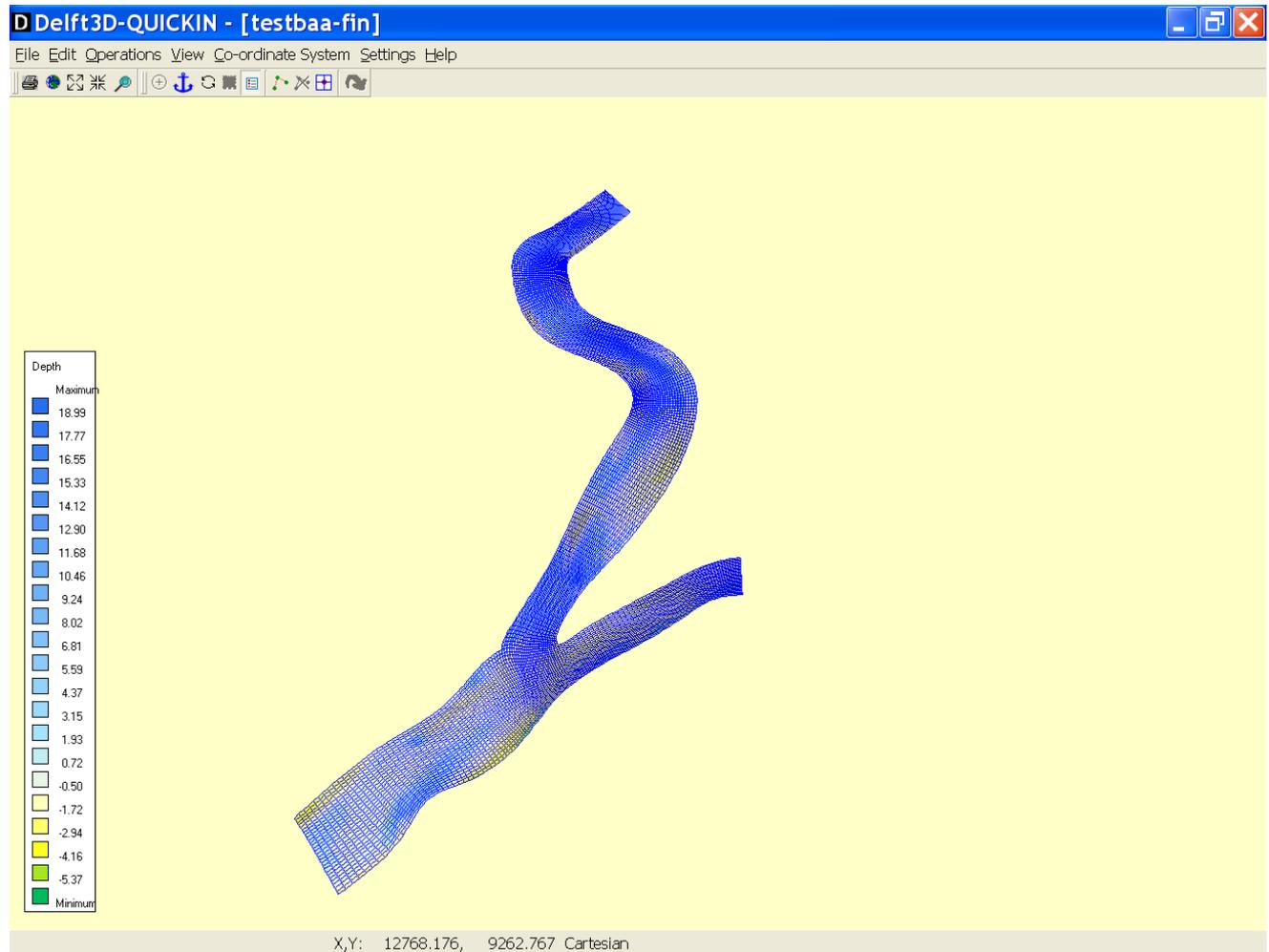
**Figure 3.1.J.9 - Computing network with bathymetric on Bala area**
