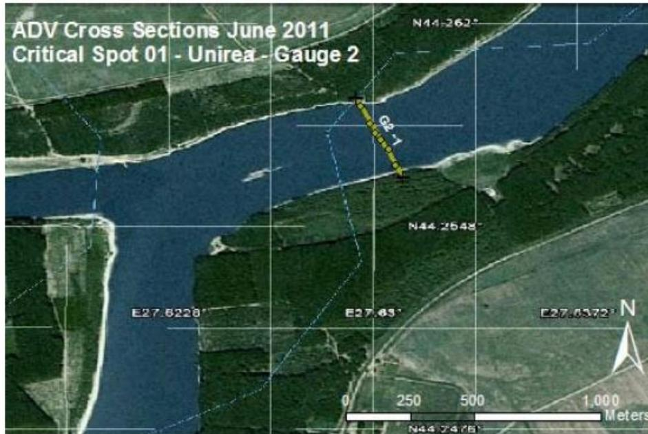
Figure 3.1.D.1.3.4 - The ADV cross sections position - Unirea area
