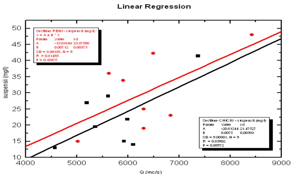
Figure 3.3.1 -  $C_{susp} = f(Q \text{ m}^3/\text{s})$  correlation at Chiciu - Silistra and Reni sections (1998 - 2009 period)
