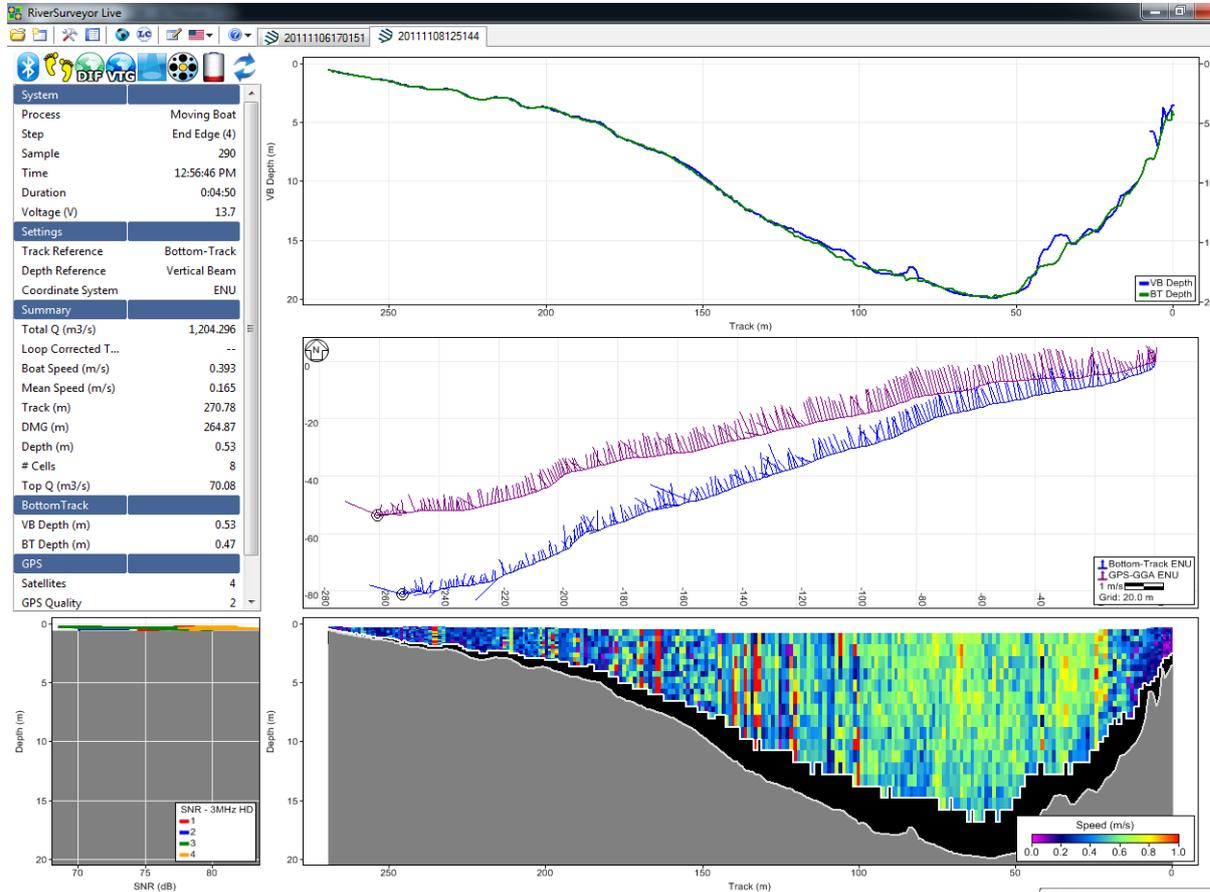
**Figure 3.1.D.1.3.1 - ADCP profile processed with River Surveyor Live software**
