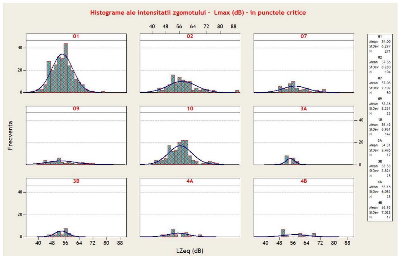
**Figure 3.1.B.1 -  $L_{max}$  (dB) noise intensity histograms**
