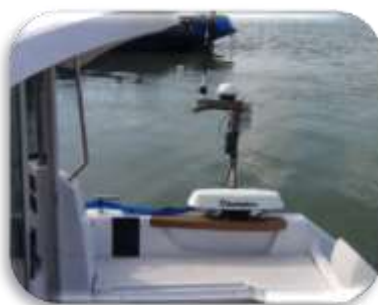
Sistem batimetric 3D Kongsberg GeoSwat Plus, 250 kHz
