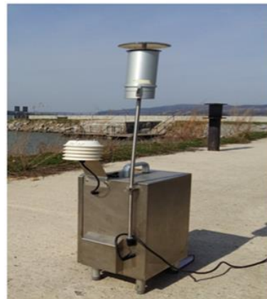
Prelevator activ tip Low Volume Air Sampler, măsurare PM1
