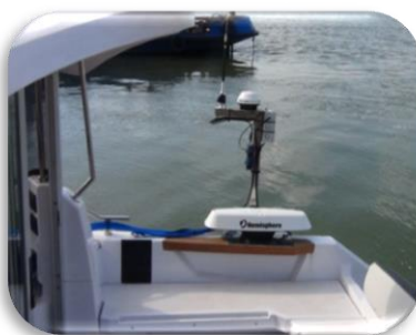
Sistem batimetric 3D Kongsberg GeoSwat Plus, 250 kHz
