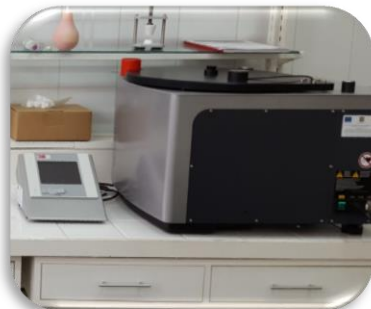
Sistem de digestie Speedwave Four, Berghouf
