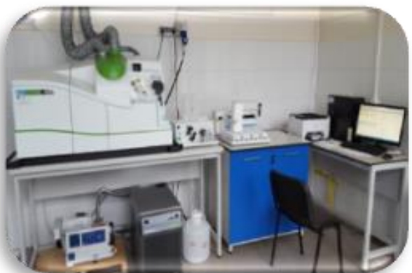
Sistem ICP-MS (Inductively Coupled Plasma - Mass Spectrometer) Nexlon 350 - Perkin Elmer
