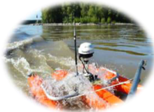
RiverRay ADCP for flow-speed measurement
