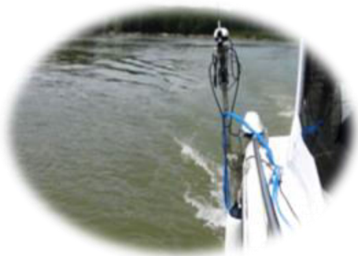
Multibathymetric system Kongsberg GeoSwat Plus Compact mounted on Ranieri CLF22 Craft
