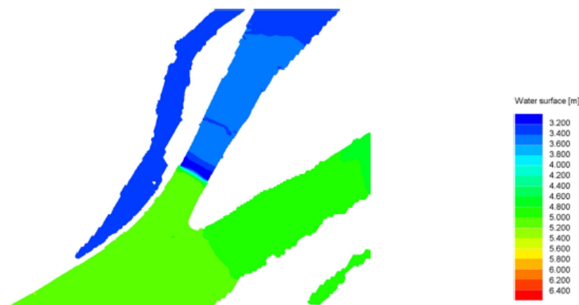
Fig. 3.1 RSim-3D results – Sill Phase III with cover and dredging– CP01 – water surface (m a.s.l.) – Q1940 \text{ m}^3/\text{s}^{-1}
